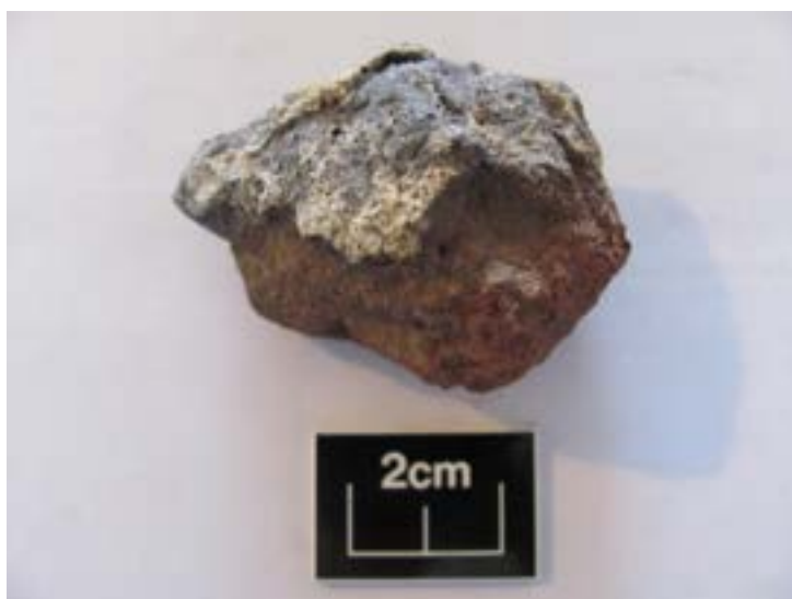
Fig. 36: Type 1 brick showing ash encrusting.
